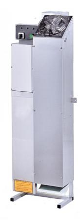
Heat and humidity generator designed for final proofing cabinets. It features a manual thermostat and hygrostat for automatic control of temperature and humidity in the fermentation cabinet. Bakers can prioritize either heat or humidity by adjusting it on the control panel
